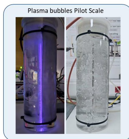
Figure 1. Photographs of the pilot-scale nanopulsed plasma bubble reactor during pollutant degradation experiments: with the stainless-steel grid serving as the grounded electrode, and without the grid, presented for illustrative purposes to highlight bubble formation.
