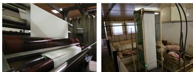
Figure 1. Production of the adsorber textile on industrial scale (left) and first prototype for the removal of ammonia in pigsties (right).
