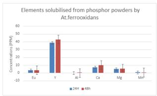
As seen in figure two low pH leaching of the phosphor powder material yielded a wider array of elements solubilized including large quantities of Europium and Yttrium as reported previous publications. Additionally small concentrations of Aluminium, Calcium magnesium and manganese were detected. No statistically significant shift in metal concentration was recorded between the two timepoints measured.
