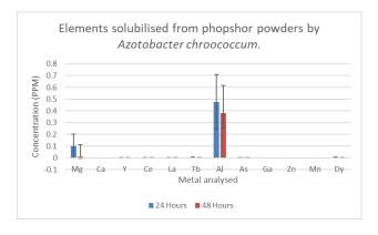
**Figure 1.** concentration of metals solubilized during 48 hours of leaching under high pH biogenic ammonia leaching
