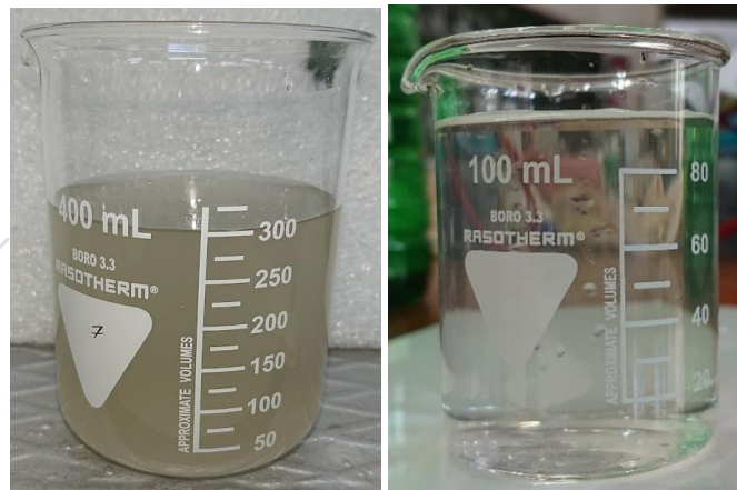
Figure 4. Water samples after filtration: without (left) and with (right) previous settling
